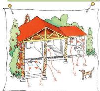
Radon moves from the soil and into your home through cracks and openings in the foundation.
